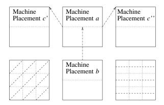
Figure 1: A depiction of six machine placements. Vertical sequencing requires that at least 50% of machine placement a be mined before beginning to mine machine placement b. Horizontal sequencing requires that machine placements c' and c'' begin to be mined once 50% of machine placement a is mined. Dotted lines divide the machine placements in the lower corners into nine production blocks each, with dashed drawdown lines at either a 45-degree angle or parallel to the surface.
