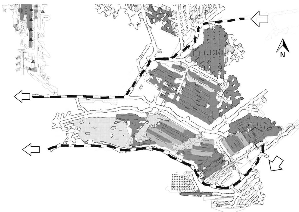
Figure 7: In this example of critical haulage routes, the dashed lines show haulage routes through a mining zone. These haulage routes are bordered by major panels containing blocks that are candidates for extraction. The pillars that support these haulage routes often consist of valuable ore blocks. However, once removed, we lose access to the area east of the extracted pillar.
