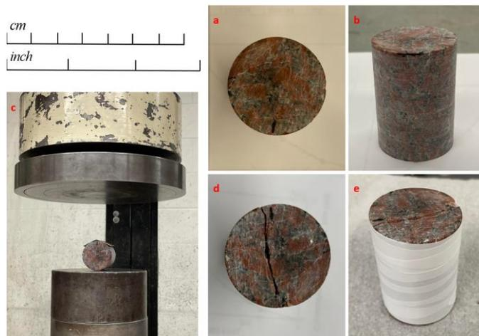
Fig. 4: Granite sample GC2: (a) top view and (b) side view prior to fracturing (these images are consistent with the scale on the left); (c) the sample and MTS machine to create a fracture; (d) top view and (e) side view of the fractured core while the core is wrapped with Teflon tape to keep core intact.
