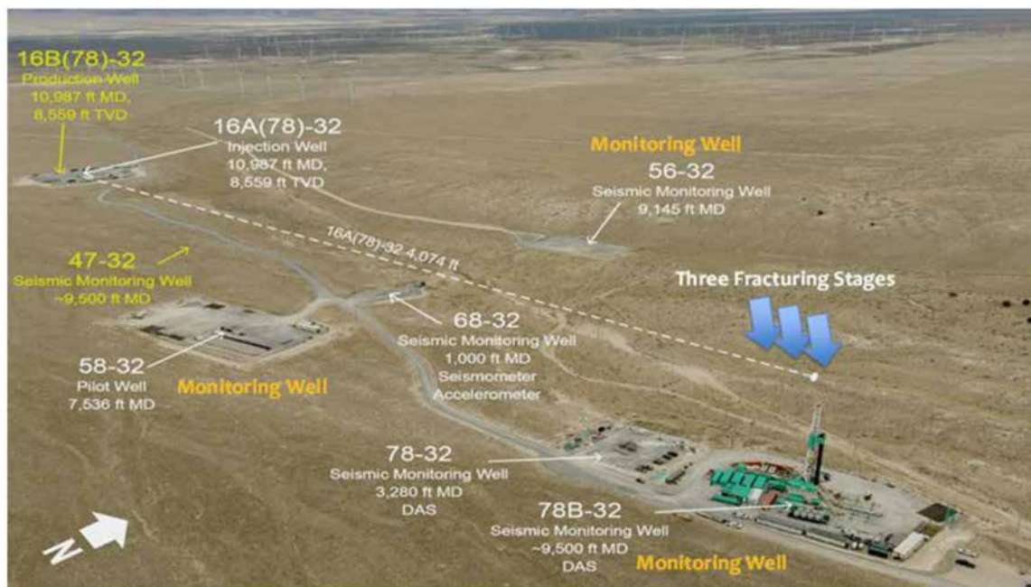
Figure 2-C—Aerial view of the wells drilled at the Utah FORGE site and the location of the three frac stages. (Source: UTAH FORGE, U.S. DOE)
