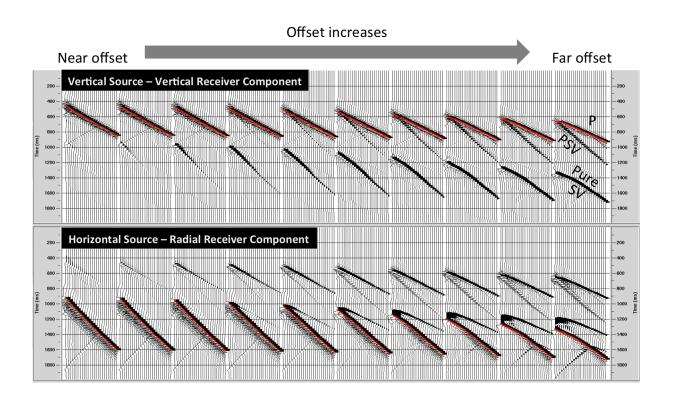
Fig. 5: Ten examples (out of 61) of the recorded vertical displacement component from a vertical source (top) and the radial component from a horizontal source (bottom). The source offset increases from left to right. See the caption of Fig. 4 for the recording geometry.
