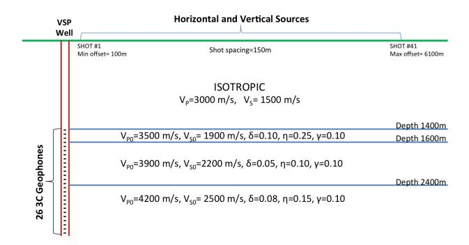
Fig. 4: Model used to generate 9C VSP data. The three bottom layers are VTI and the near-surface layer is isotropic. The density for all layers is equal to  $2.28~\rm g/cc$ . Horizontal and vertical sources (point forces) are deployed every 150 m at distances from 100 m to 6100 m away from the well. The data are recorded by 26 geophones placed in the borehole between 1400 m and 2900 m with a 60 m spacing.
