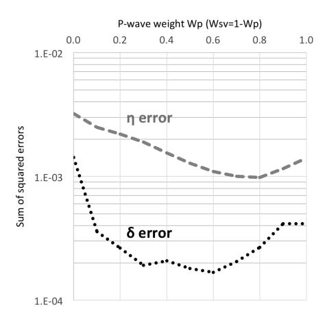
Fig. 10: Summary of estimation errors in  $\delta$  and  $\eta$  for different  $W_P$  and  $W_{SV}$  combinations and the entire VSP interval.
