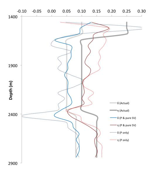
Fig. 8: Estimated parameters  $\delta$  and  $\eta$  along the well. The results of inverting solely P-waves are marked by dotted lines and of the joint inversion of P and pure SV data by solid lines. The actual  $\delta$ - and  $\eta$ -values (using a 3-geophone averaging window) are marked by light thick lines.
