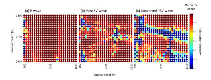
Fig. 6: Linearity of the particle motion for P-waves, pure SV-waves and converted PSV-waves. Unity corresponds to a linear particle motion, while zero means that the particle motion is circular.
