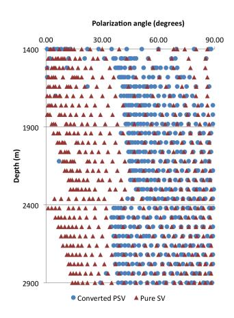
Fig. 12: Polarization angles of pure SV- and converted PSV-waves used in the joint inversion.
