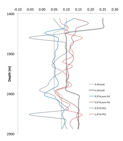
Fig. 11: Parameters  $\delta$  and  $\eta$  estimated using P- and converted PSV-wave data (dotted lines) and P- and pure SV-waves (solid lines). The actual  $\delta$  and  $\eta$  values (using a 3-geophone averaging window) are marked by light thick lines.
