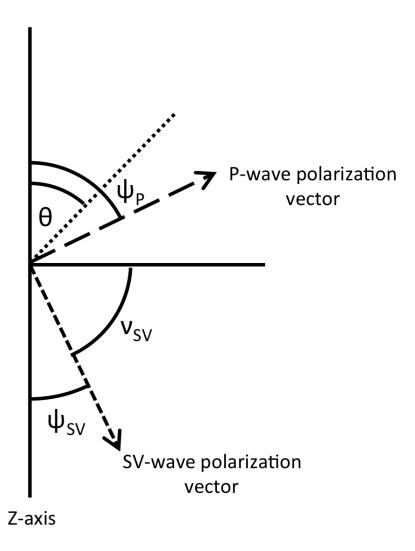
Fig. 13: Diagram of the angles used in the derivation. The phase angle  $(\theta)$  of both Pand SV-waves, P-wave polarization angle  $(\psi_P)$ , SV-wave polarization angle  $(\psi_{SV})$ , and the angle  $\nu_{SV}$  between the SV-wave polarization vector and the horizontal.
