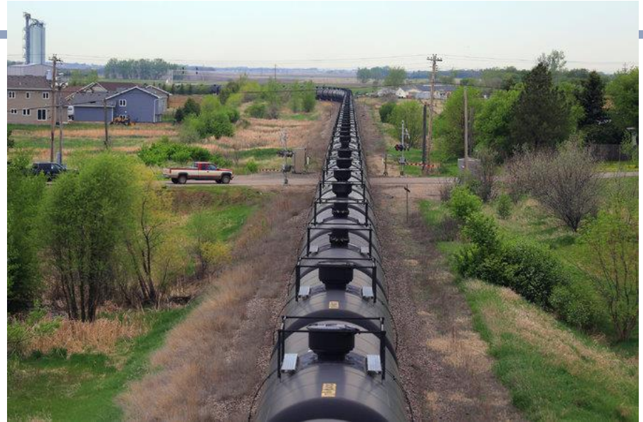
Each rail car holds about 30,000 gal (714 bbls)
