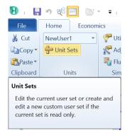
In the lower section let's start with the *refining* unit set. Select refining & press Copy. A new unit set will be created (here called NewUser2). Double click on this name & enter Refining-US.
