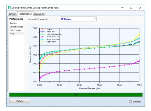
You can also create a Stream Analysis by rightclicking a stream & picking the appropriate option. For example, right-clicking on the Diesel stream can get you to the option shown & will create a set of boiling point curves.
