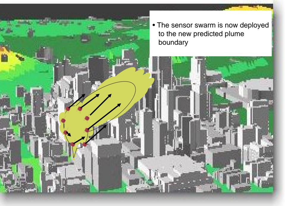
• The sensor swarm is now deployed to the new predicted plume boundary, where new samples are taken.
