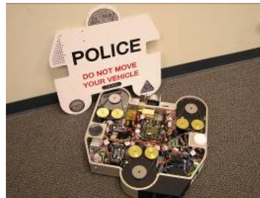
Fuel-cell powered ODIS developed by Kuchera Defense Systems
