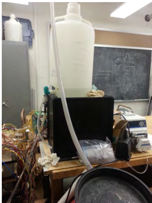
(a) Constant head reservoir being fed by ground reservoir (required due to volume of water)
