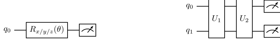
Figure 2.1 Examples of two quantum circuits. (left) A single qubit rotation gate in the x, y or z basis with angle \theta , followed by a measurement gate. (right) a general two-qubit quantum circuit for two unitary applications U_1 and U_2 , followed by two single qubit measurement gates.
